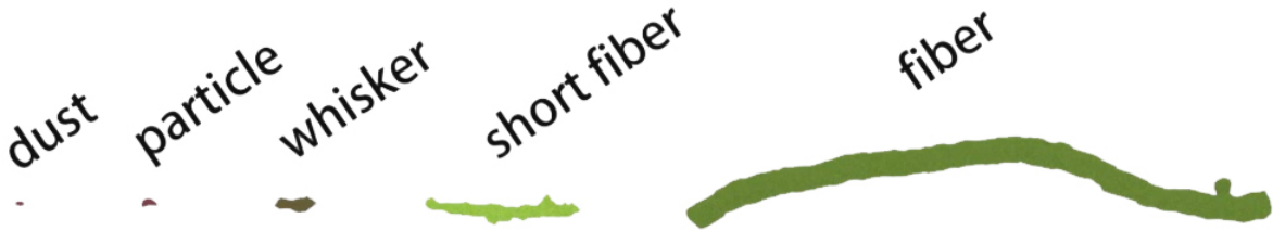
FIGURE 3 – Different short fiber morphologies identified with clustering.
